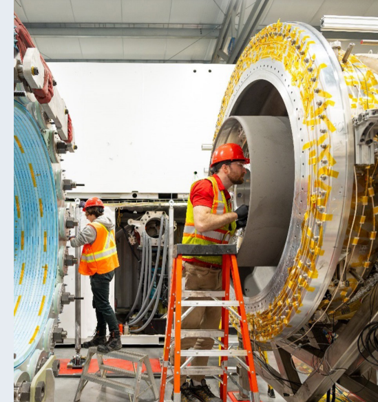
For LM26, General Fusion integrated its operational plasma injector with a compression system
